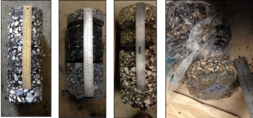
Figure 10 – Core degradation, Left to right: good, medium, severe, very severe (rubble in bag)
